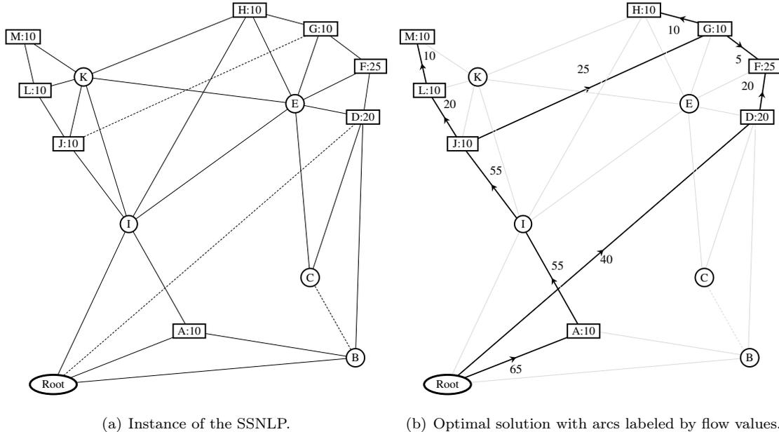
Figure 1: Graph  $G = (V, E)$  with  $|V| = 14$ , euclidean edge lengths and  $|\mathcal{N}_e| = 1$ , for all  $e \in E$ . Solid lines are edges that allow the cable type:  $(u_{e,1}, c_{e,1}) = (100, 120)$  (e.g., street-connections). Dashed edges allow the cable type:  $(u_{e,1}, c_{e,1}) = (40, 10)$  (e.g., existing infrastructure). Rectangle nodes are customers with their demands written at the corresponding labels.
